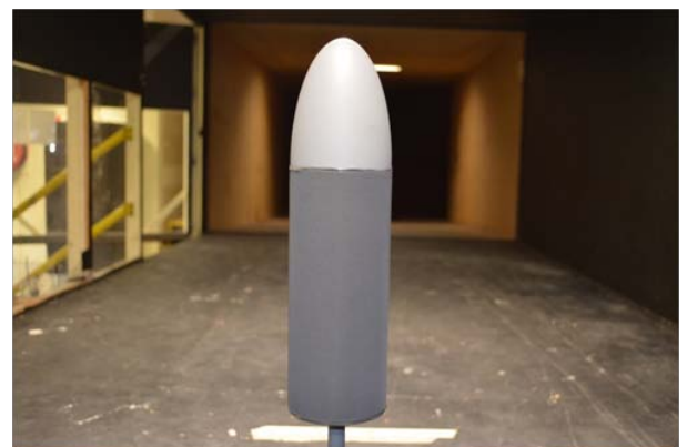
Fig.3: Test cylinder fitted with fabric sample
